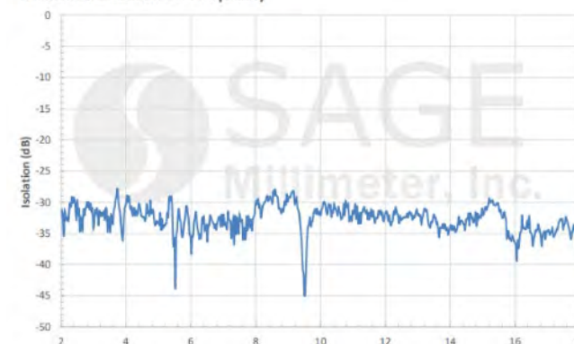
Measured Isolation vs. Frequency
