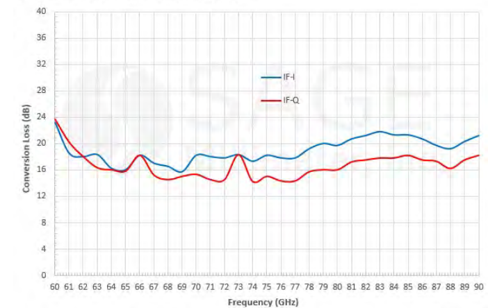
Typical Conversion Loss vs. Frequency
